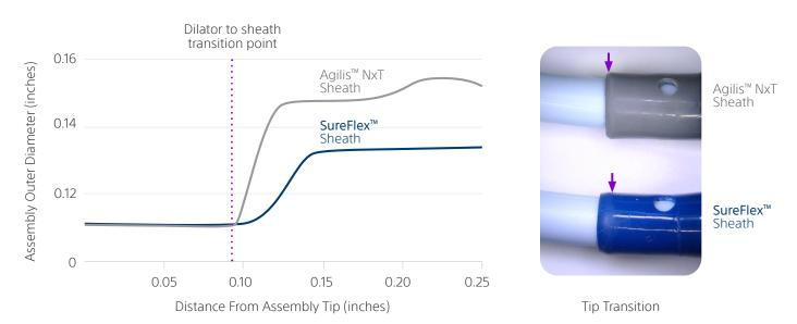
Figure 2. Dilator-to-sheath transition comparison (left: outer diameter measurements; right: device photographs)
